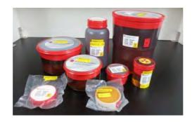
As shown in Fig. 2 (a, b), these samples includes soil, water, plant, food, dust in the atmosphere, filtered substance, etc. Measured sample, except for the dust and filtered substance, is packed in a plastic container with predetermined shape.
