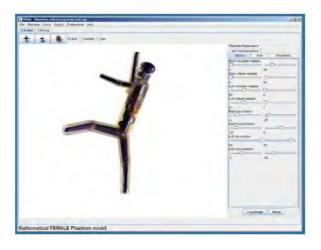
Figure 2 shows the "Simulation" tab in the right plane that allows various parameters to be set for the simulation. This allows the novice MCNP user to insert various source configurations to the input file, and permits experienced MCNP users to manually modify the generated input file with custom preferences.
